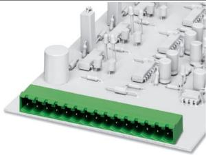
Header, nominal current: 12 A, rated voltage: 250 V, pitch: 5.08 mm, no. of positions: 12, mounting: Soldering
